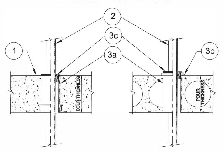
1. Floor: Minimum 4-1/2" thick normal density concrete slab or 7-1/2" thick hollowcore precast concrete floor units. Fluted decks with 2-1/2" concrete slab, rating is 1Hr F/FH
