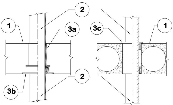
**1. FLOOR:** Minimum 4-1/2" thick normal density concrete slab. Fluted decks with 2-1/2" concrete slab, rating is 1Hr F/FH Or (Floor Only) 7-1/2" thick hollowcore precast concrete units. Minimum 6" thick classified block or normal density concrete.
