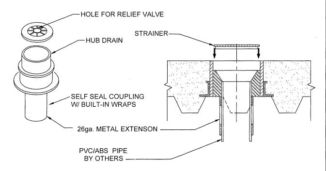
USED FOR CONDENSATE TYPE DRAINS
