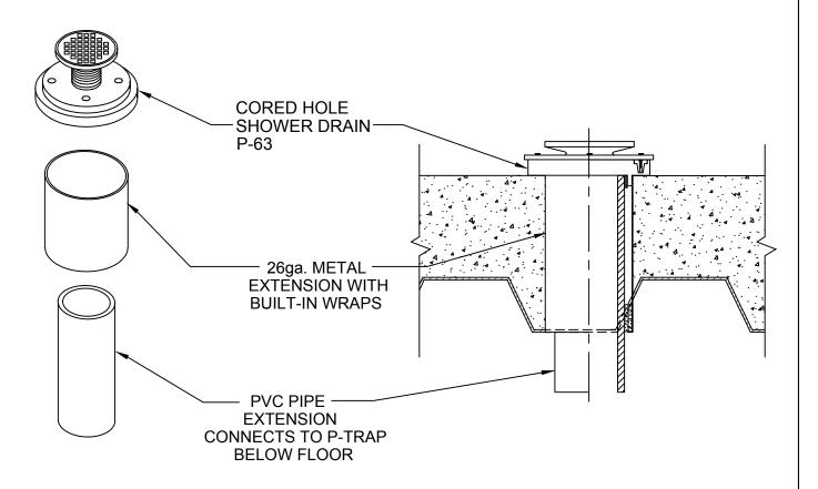
SEE COMPONENT DETAIL P-63 FOR VARIOUS SIZE STRAINER OPTIONS. SEE DRAWING C-6330-A-B FOR CAST-IN PLACE & C-6330-C FOR METAL DECK.
