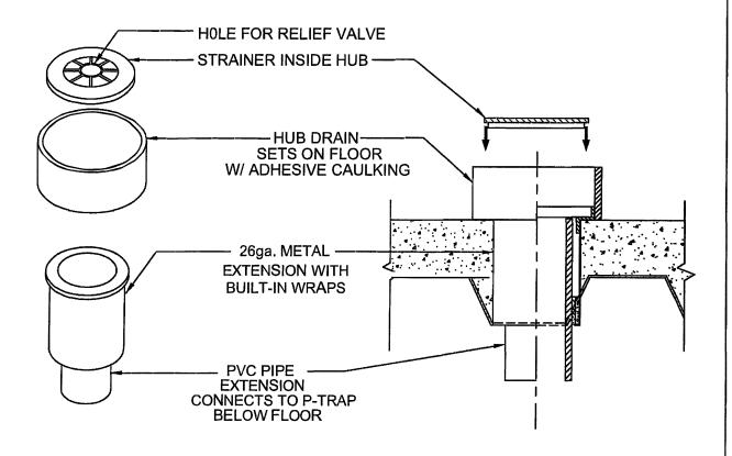
SEE DRAWINGS C-6320-A & B FOR INSTALLATION IN POURED IN PLACE CONCRETE FLOORS.
