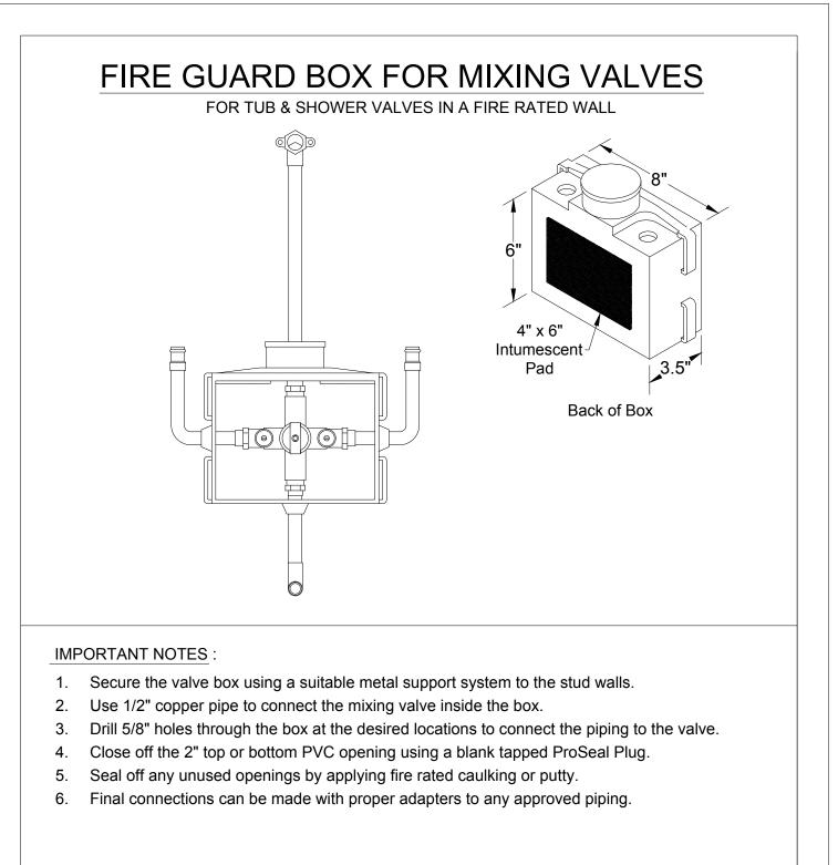
Reversing the valve box installation is optional
