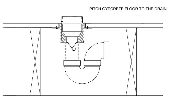
MOUNT FLANGE FROM THE TOP WITH GYPCRETE FROM THE BOTTOM WITHOUT USE T-3SO STRAINER WHEN DISCHARHING A RELIEF VALVE INTO THE HUB DRAIN
