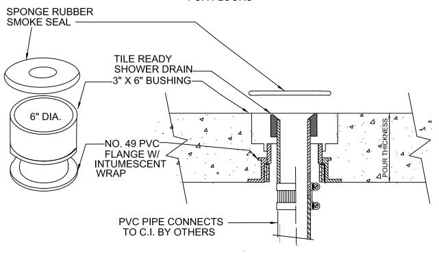
SEE DRAWING T-6330-C FOR METAL DECKS & T-6330-D FOR CORED HOLES.
