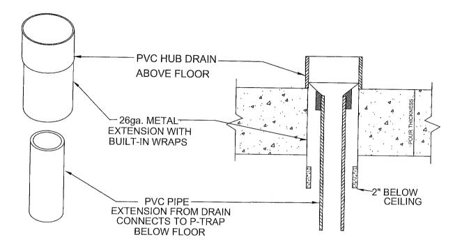
SEE DRAWING T-6330-A FOR CAST-IN PLACE & T-6330-CPS FOR METAL DECK.
