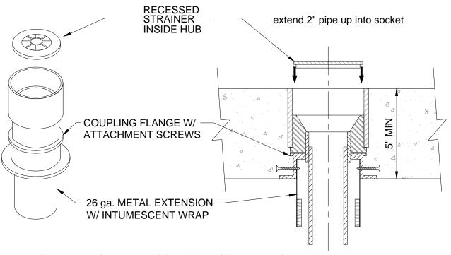
STRAINER CAN BE FLUSH WITH FLOOR FOR FLOOR DRAIN OR RECESSED 1-1/4" INTO HUB FOR COMBO HUB/FLOOR DRAIN
