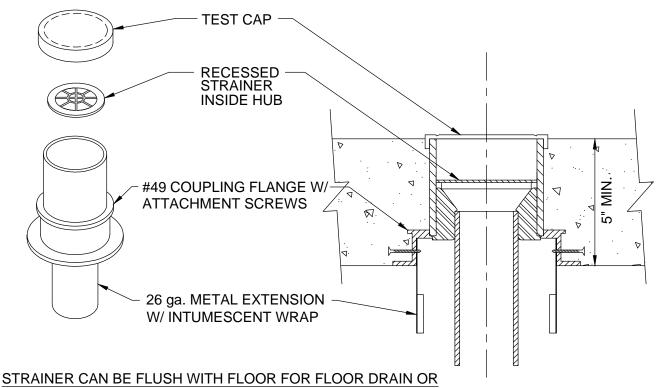
STRAINER CAN BE FLUSH WITH FLOOR FOR FLOOR DRAIN O
