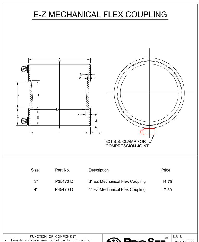
Female ends are mechanical joints, connecting similar & dissimilar pipe materials.
