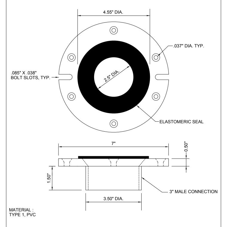
\* FUNCTION OF COMPONENT Used to fit inside a 3" closet stub hub end.
