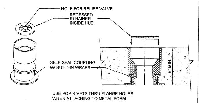
STRAINER CAN BE FLUSH WITH FLOOR FOR FLOOR DRAIN OR RECESSED 1-1/4" INTO HUB FOR COMBO HUB/FLOOR DRAIN
