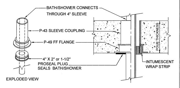
THIS SPECIAL PENETRATION ISD USED TO PROVIDE MOVEMENT WITH A LARGER OPENING TO CONNECT PRECAST BATH TUBS AND SHOWER BASES.
