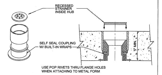
STRAINER CAN BE FLUSH WITH FLOOR FOR FLOOR DRAIN OR RECESSED 1-1/4" INTO HUB FOR COMBO HUB/FLOOR DRAIN
