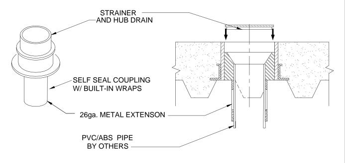
USED FOR CONDENSATE TYPE DRAINS
