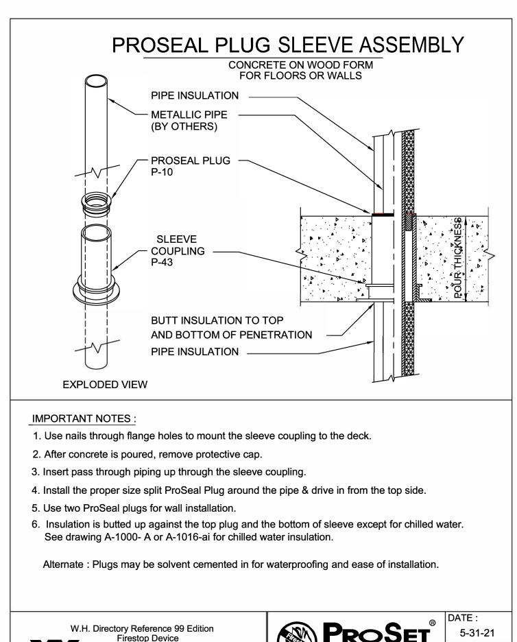
W.H. Design No. PS/PHV 120-03 F Rating 2 Hrs.or 3 Hrs or 4 Hrs
