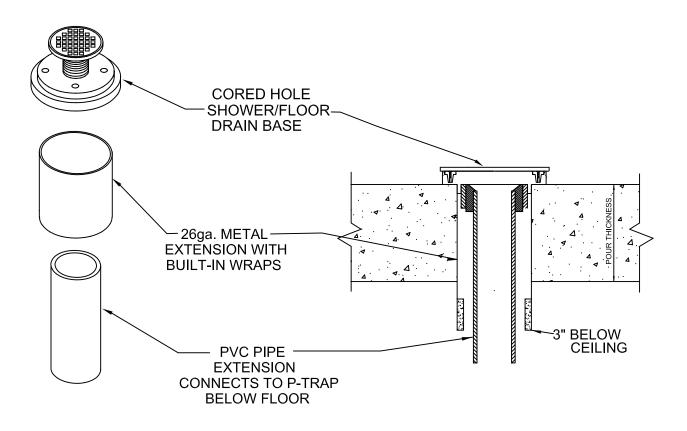
SEE T-RITE STRAINER TOPS FOR VARIOUS TYPES AND SIZE STRAINER OPTIONS. SEE DRAWING T-6330-A FOR CAST-IN PLACE & T-6330-C FOR METAL DECK.
