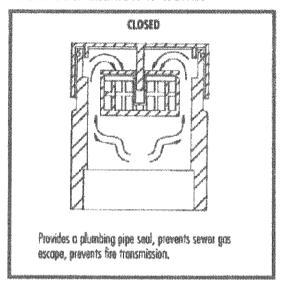
The combination Firestop Device and Plumbing Vent can be used through fire rated floors and walls. The floors can be poured or cored concrete or wood floor/ceiling assemblies. The Air Vent Fire Tests were conducted by Warnock Hersey and are listed in their Fire Resistance Directory under design numbers PS/PH 120-08 and 120-09.
