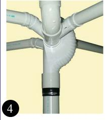
After inserting the pipe into the rolled back E-Z Flex, pull the bottom flex portion of the coupling back down around the pipe and tighten the clamps to complete the installation.
