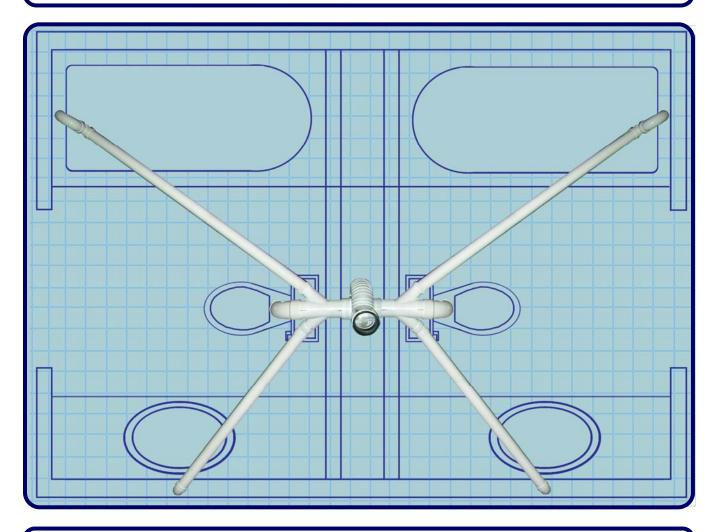
Picking up the lavatory underneath the slab eliminates the need to drill through all the stud walls. The top rough will be completed without any walls. The sleeves support the pipes without using regular hangers. The bath tub waste connects to ProSet's tub box.
