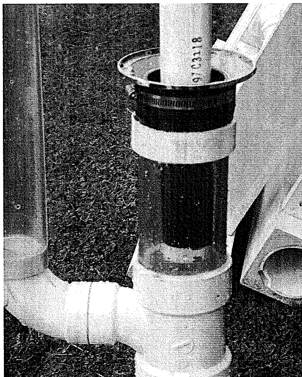
PHOTOGRAPH 16 1 1/2-INCH PVC PIPE INSERTED
