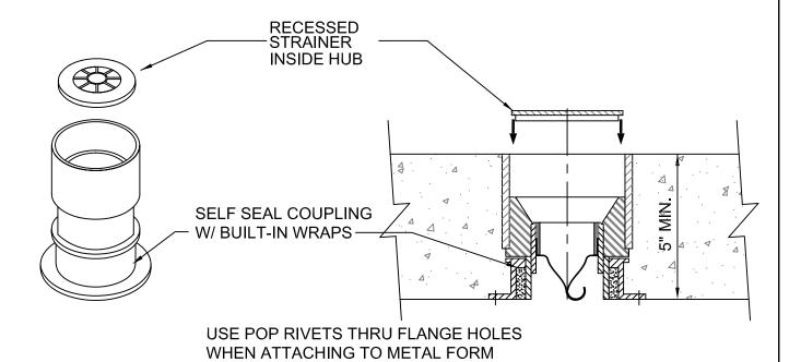
STRAINER CAN BE FLUSH WITH FLOOR FOR FLOOR DRAIN OR RECESSED 1-1/4" INTO HUB FOR COMBO HUB/FLOOR DRAIN
