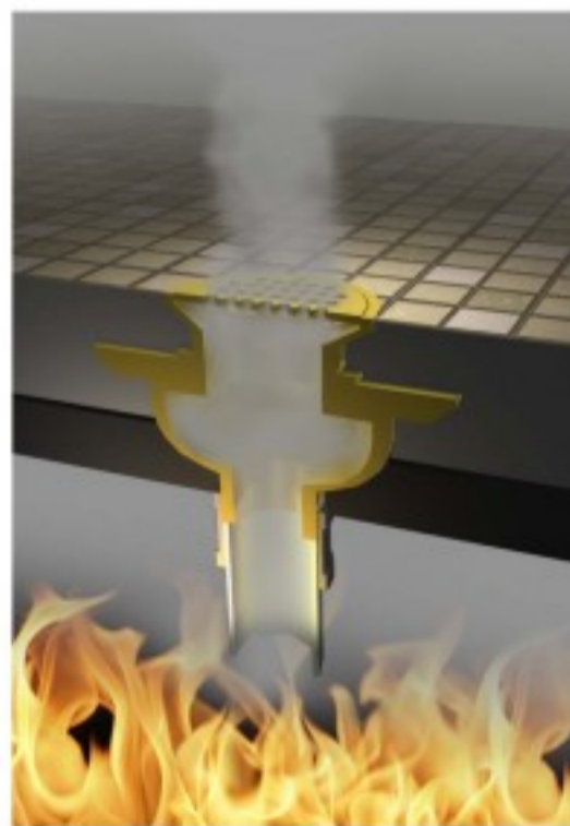
figure 1: Regular firestopping allows toxic smoke transmission
