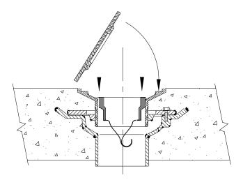
PART NO. TG33-WADE 3" INSERT FITS INSIDE 1100 3" & 4" DRAINS DRAINS FOR TRAP GUARDS FITTING INTO GASKET CONNECTED DRAINS, SEE DRAWING TG-23-G
