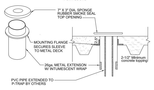
SEE DRAWINGS T-6300-APS FOR CONCRETE ON WOOD FORMS & T-6300-DPS FOR CORED HOLE
