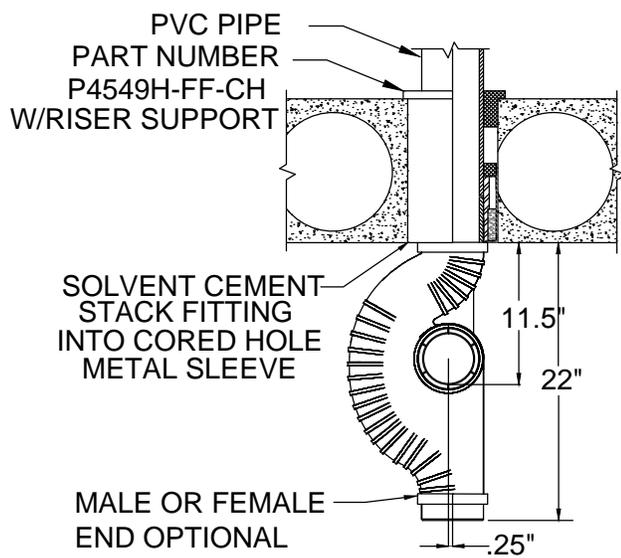
4" x 3" STACK INTO A CORED HOLE SLEEVE
